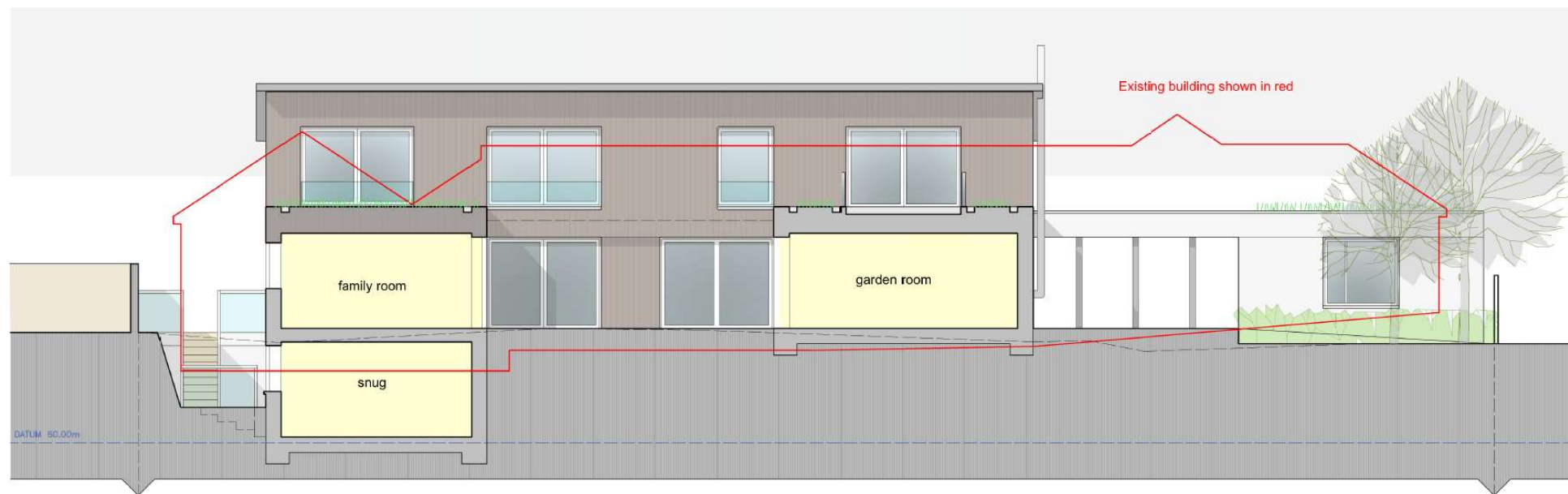
Proposed section BB scale 1:100 @A3 See drawing 10 for section references
